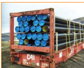
One of the 4 x 40 foot Flat-rack sea containers
